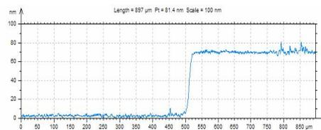
**Figure 4:** ARC thickness measurement obtained using the ASIQ.
