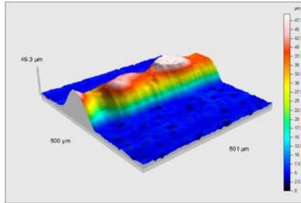
**Figure 6:** 3D plot of an electrical contact line.
