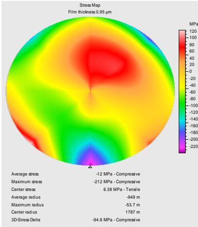
**Figure 5:** Typical 3D stress measurement after film deposition.
