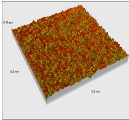
**Figure 3:** 3D plot of a Solar Cell after the roughening process.
